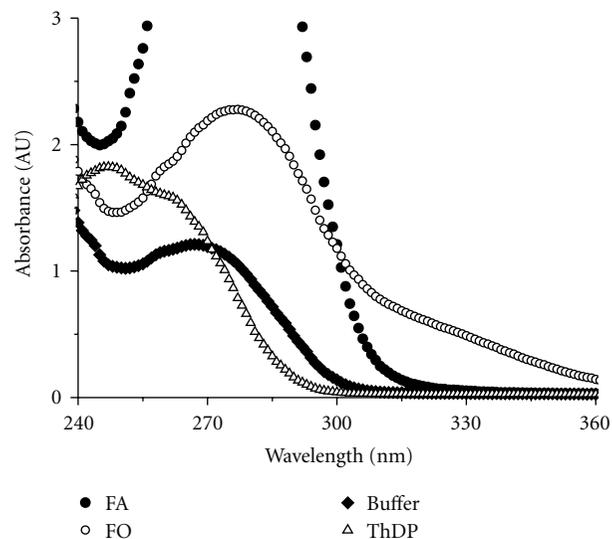
FIGURE 2: Spectra of substrate (●; FA, furaldehyde  $0.7 \text{ mmol L}^{-1}$ ), product (○; FO, Furoin  $0.33 \text{ mmol L}^{-1}$ ), buffer with ThDP (◆)  $0.25 \text{ mmol L}^{-1}$ , and only ThDP (△)  $0.25 \text{ mmol L}^{-1}$  in water.
