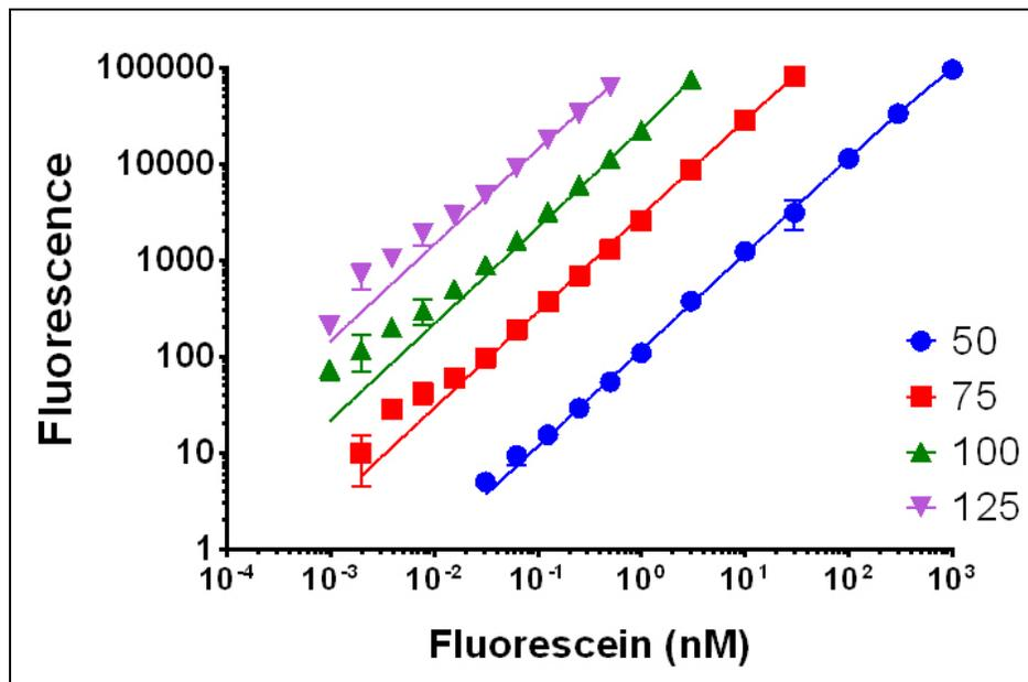
**Figure 6. Fluorescein titration measured using fixed gain.** The fluorescence signal at different PMT gain settings from a single sodium fluorescein titration was graphed using Log scale axis. Data represents the mean and standard deviation of 4 determinations at each concentration.
