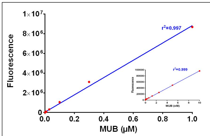
**Figure 7. 4-Methylumbelliferone titration measured using extended dynamic range.** The linear regression analysis of fluorescence from 0 to 1  $\mu\text{M}$  concentrations of MUB was plotted on linear axis. Inset depicts results for low concentrations (0-10 nM) of MUB. Data represents the mean and standard deviation of 4 determinations at each concentration, with  $r^2$  values of each linear regression shown.
