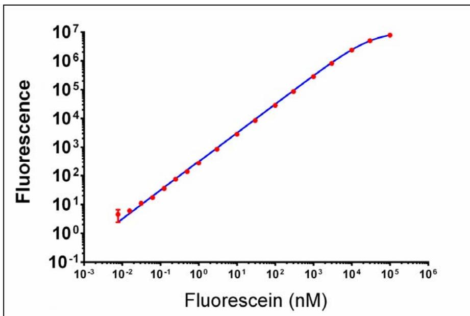
**Figure 5. Fluorescein titration measured using extended dynamic range.** Log-log plot of fluorescence from a sodium fluorescein titration. Data represents the mean and standard deviation of 4 determinations at each concentration.
