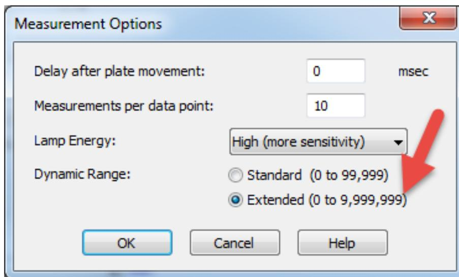
**Figure 3. Selection of the extended dynamic range button in the Measurements Options Window.** Among the number of read parameters can be altered is the Dynamic range, where Standard and Extended dynamic range are available.
