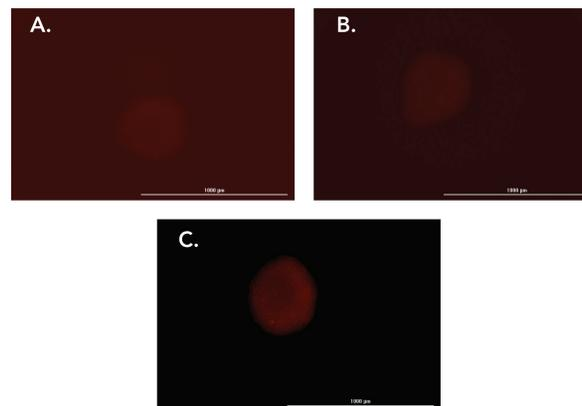
**Figure 2.** 4x images of Hypoxia Red Reagent signal captured after (A) 2 hours; (B) 4 hours; and (C) 6 hours of incubation with the spheroid at 37 °C/5% CO<sub>2</sub>.
