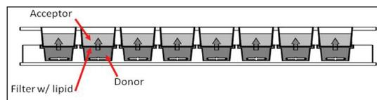
**Figure 2.** Cross-section of PAMPA Explorer™ sandwich plate: compound is loaded into Donor compartment and allowed to passively (with stirring) pass through the filter with lipid (artificial membrane) over a defined time period. Permeability is determined by measuring the absorbance of compound in the Donor and Acceptor compartment and comparing them to the initial compound's absorbance.
