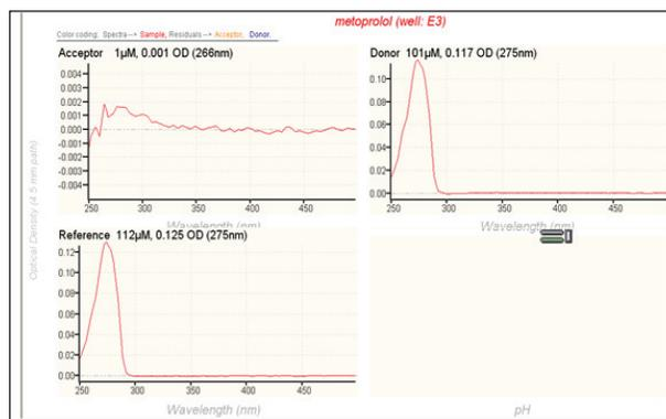
**Figure 5.** Detailed view of PAMPA Explorer software measuring absorbance spectra from metoprolol in Donor compartment, as a reference solution and from the Acceptor compartment demonstrating the permeability of the compound through the PAMPA membrane.
