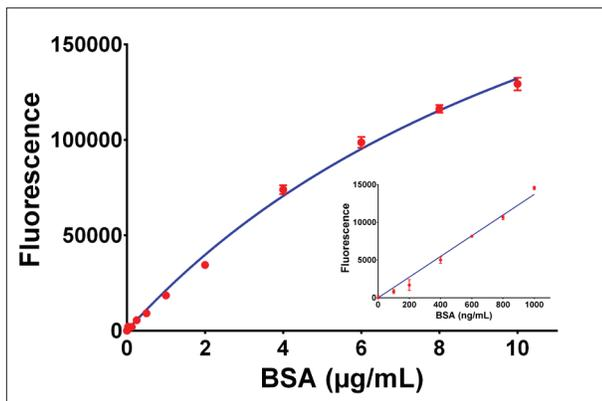
**Figure 2. Linearity of Monochromator-based Detection.** Concentration curve from 0.0 to 10  $\mu\text{g/mL}$  of BSA with 4-parameter regression analysis. Insert figure depicts the data points for the lower concentrations (0 to 1000 ng/mL) with a linear regression analysis. Data points represent the mean values of eight determinations at each concentration.
