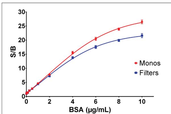
**Figure 3. Signal/Background Comparison of Monochromator- and Filter-based Detection.** The ratio of each sample to the mean of the blank (0  $\mu\text{g/mL}$  BSA) was plotted. Data represents the mean and standard deviation of eight determinations.
