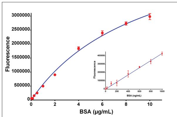
**Figure 1. Linearity of Filter-based Detection.** Concentration curve from 0.0 to 10  $\mu\text{g/mL}$  of BSA with 4-parameter regression analysis. Insert figure depicts the data points for the lower protein concentrations (0 to 1000 ng/mL) with a linear regression analysis. Data points represent the mean values of eight determinations at each concentration.
