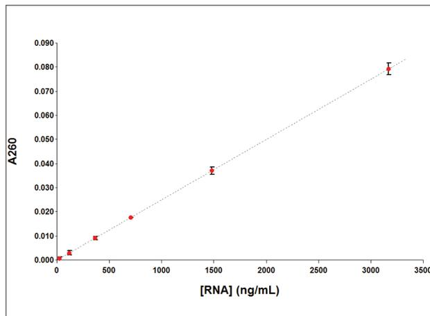
**Figure 1.** RNA absorbance measurements. A dilution series of ribosomal RNA was prepared ranging from 0 – 3,200 ng/mL in TE buffer. Standards were analyzed in triplicate at a volume of 100  $\mu$ L in a UV transparent, 96-well microplate format.
