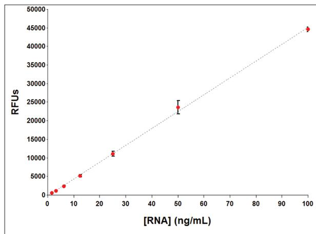
**Figure 3.** Low range measurements. A dilution series of ribosomal RNA was prepared ranging from 0 – 100 ng/mL in TE buffer. Standards were analyzed in triplicate at a volume of 100  $\mu$ L in a standard 96-well microplate format.
