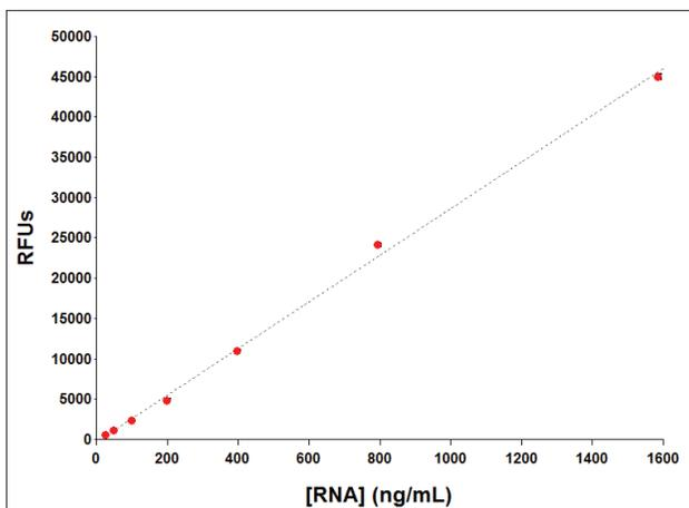
**Figure 2.** High range fluorescence measurements. A dilution series of ribosomal RNA was prepared ranging from 0 – 3,200 ng/mL in TE buffer. Standards were analyzed in triplicate at a volume of 100  $\mu$ L in a standard 96-well microplate format.
