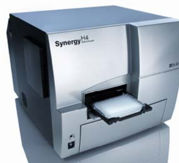
Figure 1. Synergy™ H4 Hybrid Multi-Mode Microplate Reader. The instrument was used to quantify the fluorescent signal from all assay plates, as well as perform spectral scanning.
