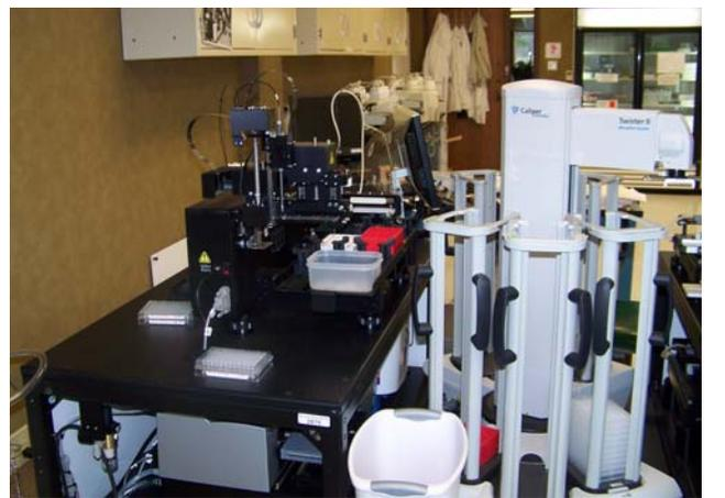
**Figure 5. Left Side View of System.** The Twister II robotic arm/gripper and storage racks are seen in the center section, while the Precision XS is seen on the top level of one of the end-unit tables.
