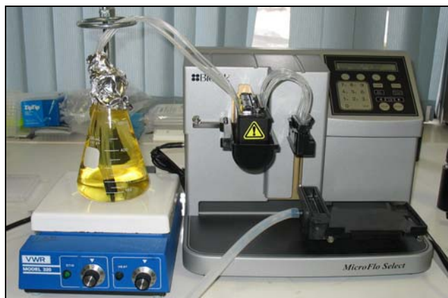
Figure 1. Instrument configuration. A MicroFlo configured with a 10 µL tubing cassette.
