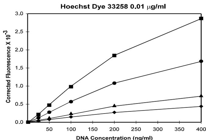
**Figure 3. The effect of 0.01 µg/ml Hoechst 33258 dye concentration on fluorescent signal.** Dilutions of DNA were made with Hoechst 33258 dye at 0.01 µg/ml. Fluorescent signal determined at four different sensitivity (u 60; s 66; l 74; n 80) settings and their fluorescent signal determined.
