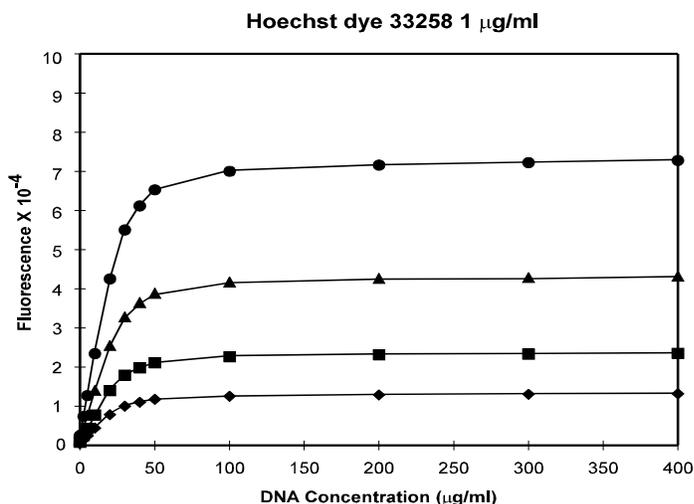
**Figure 1. The effect of 1.0 µg/ml Hoechst 33258 dye concentration on fluorescent signal.** Dilutions of DNA were made with Hoechst 33258 dye at 1 µg/ml. Fluorescent signal determined at four different sensitivity (u 44; n 48; s 52; l 56) settings and their fluorescent signal determined.
