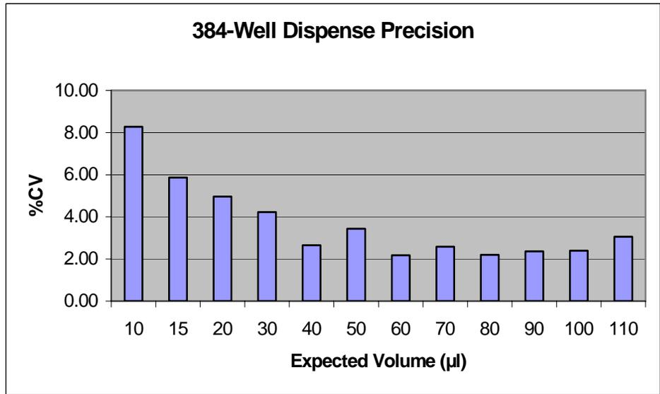
**Figure 3. Dispense Precision of the ELx405 HT.** The volume dispensed to each well was determined as described in the materials and methods. The use of a plate-specific conversion factor that allows the conversion of an absorbance measurement to volume. The mean, standard deviation and %CV were then calculated from the calculated volumes. Note that the %CV for each indicated volume represents 384-well determinations.
