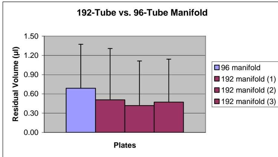
**Figure 5. Comparison of 96-well and 192-well manifold Residual Volumes.** Using the same ELx405 washer, 384-well plates containing 100 µl of concentrated blue dye were aspirated with either the standard ELx405 Select 96 tube-pair manifold or the ELx405 HT, 192 tube-pair manifold, were tested for residual liquids as described in materials and methods. Note that error bars represent the maximal residual volume in any well.
