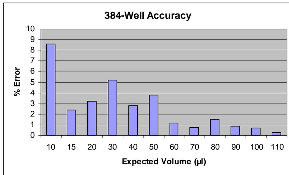
**Figure 2. Dispense Accuracy of the ELx405 HT Microplate Washer.** For each volume indicated, individual 384-well microplates were weighed. After dispensing the indicated volume using the ELx405 HT, the plates were re-weighed. The total residual volume of the plate was calculated assuming a specific gravity of 1 g/ml. The percent deviation is the ratio of the difference between the calculated and expected values to the expected values expressed as a percent.
