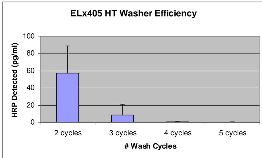
**Figure 6. ELx405 HT Washer Efficiency.** Horseradish peroxidase (HRP) enzyme was pipetted into all the wells of 384-well microplates and the plates washed with the indicated numbers of wash cycles using an ELx405 HT Microplate Washer. HRP activity was assayed after washing and activity calculated by comparison against a previously prepared standard curve. Note that each bar represents the mean and standard deviation of all the wells of a 384-well microplate.
