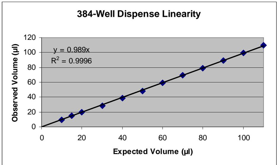
**Figure 4. Linearity of Dispense.** The calculated observed volume from data presented in Figure 3, was plotted against the corresponding expected volume. The data (blue diamonds), which represent the mean determination of 384-wells, was plotted and a linear regression analysis performed. The subsequent regression (solid line) and its equation and correlation coefficient are also presented.
