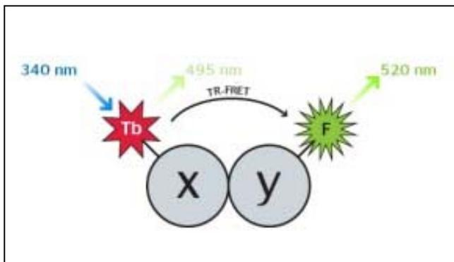
Figure 1. Principle of LanthaScreen™ TR-FRET detection.
