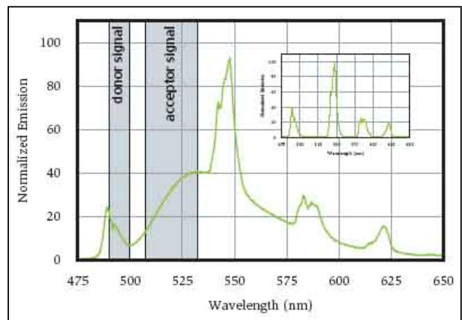
Figure 2. Fluorescence Spectra of Terbium and Fluorescein (FRET) emission. The time-resolved spectra above illustrate energy transfer occurring when terbium (donor) and fluorescein (acceptor) are brought into proximity via biomolecular interactions. The inset shows the time-resolved spectra in the absence of energy transfer.
